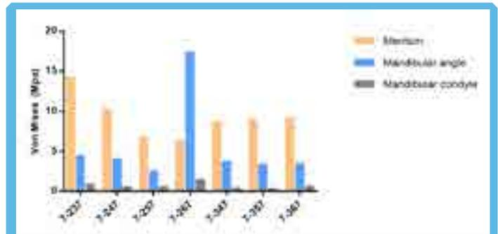
**Figure 15:** The von Mises stress value and distribution of the mandible, while repairing to the second molar.
