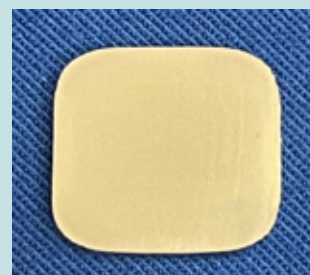
Figure 4: Ceramic wafer 12.8 X 14.8 X 1mm used.
