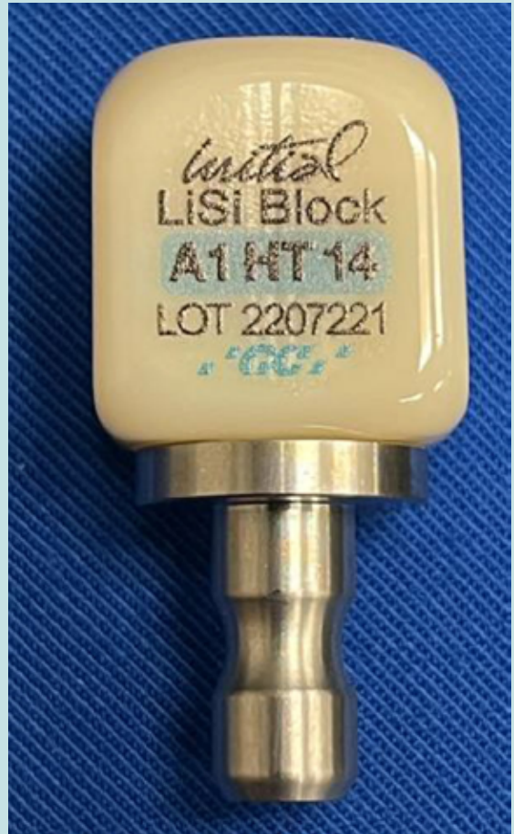
Figure 2: Initial LiSi lithium disilicate block used for ceramic wafer specimens.
