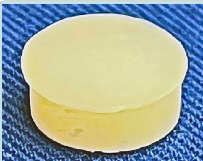
Figure 1: Bulk cement specimen 8mm X 3 mm.
