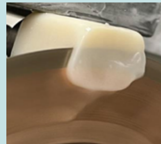
Figure 3: Preparing 1mm thick wafer from ceramic block using a diamond saw.
