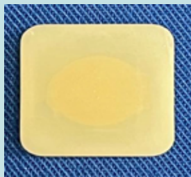
Figure 7: Final cement/wafer assembly following visible light polymerization.
