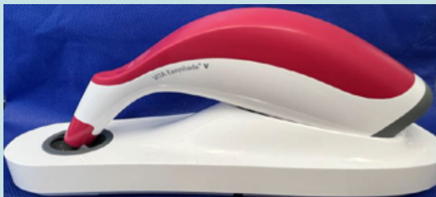
Figure 8: VITA Easyshade V device for measuring CIELAB L^*a^*b^* values.
